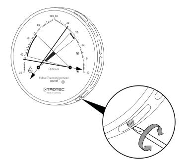
In addition, the device should be moistened once a year. This is recommended in particular after longer periods with a low humidity level. To do so, wrap the entire device into a damp, warm cloth for approx. 30 minutes. It must then display 95 to 98 %. If the pointer is not within this range, the indication must be adjusted.
