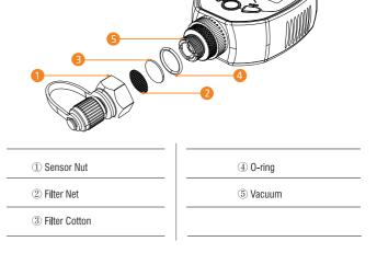
The filter cotton in the cavity is used to filter impurities and reduce sensor pollution. In order to maintain the best measurement accuracy, regular inspection is required. Follow the steps below:
