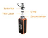
The filter cotton is used in the vacuum chamber to filter impurities and reduce sensor pollution. In order to maintain the best measurement accuracy, normal use needs to be checked every three months (adjust the inspection period according to the frequency of use). If the filter is seriously polluted, it needs to be replaced.
